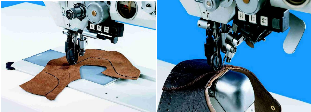
Figure 7. Different types of stitching machines. On the left the flat-bed stitching machine. On the right the pillar stitching machine
