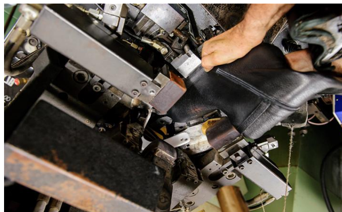
Figure 51. Roughing. Source: CTCP
