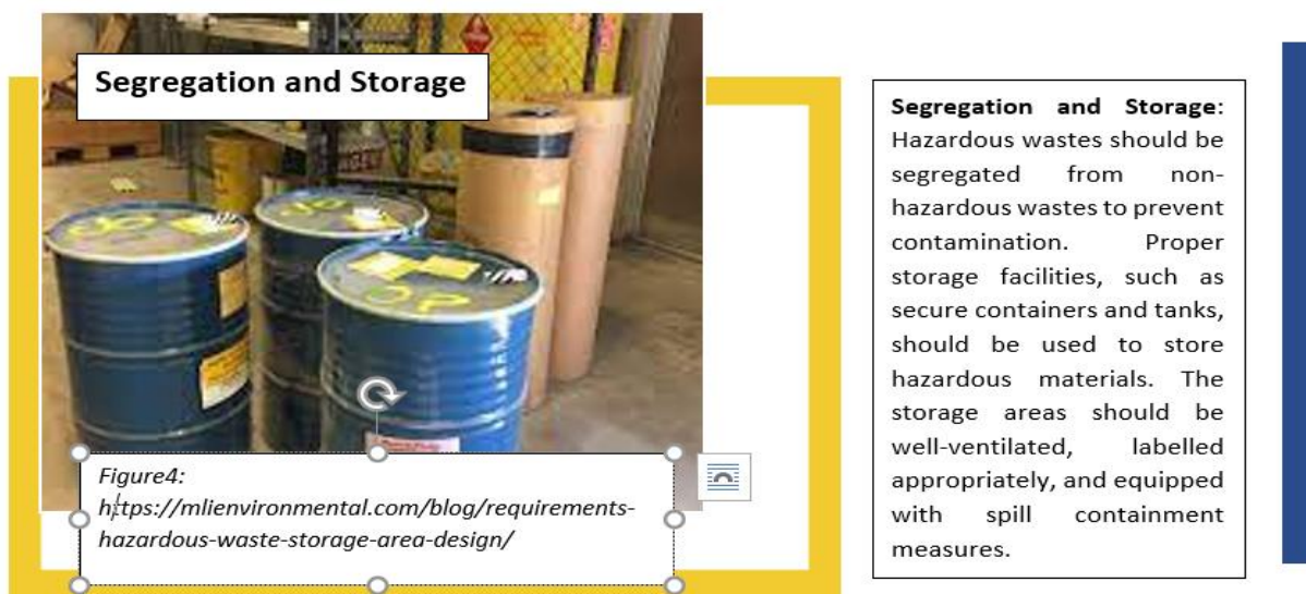
Figure 18. Segregation and storage
