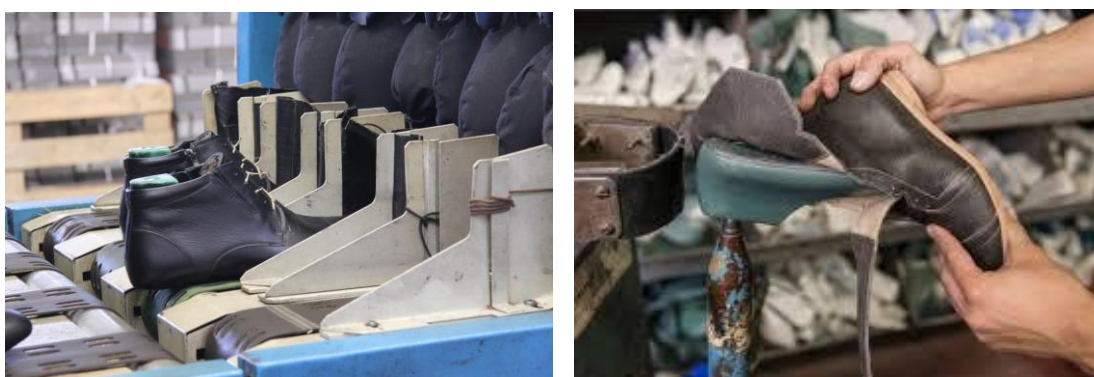
Figure 15. On the left Stabilize shoe; on the right Sslip the last on Last slipping machine
