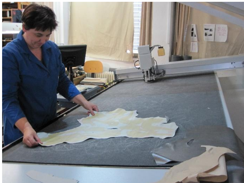
Figure 28. Automatic Cutting Machines – Semi automatic process
