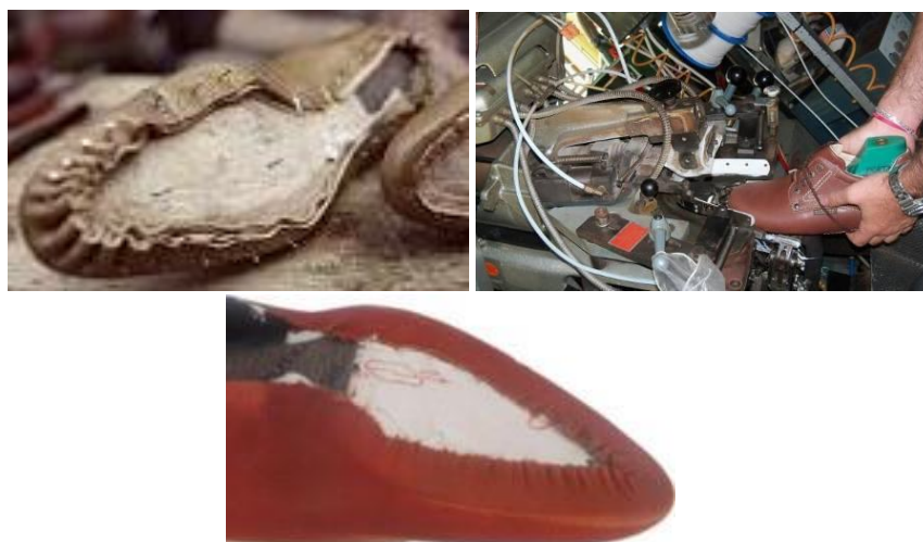
Figure 9. Assembly by hand, by machine, assembly cemented construction
