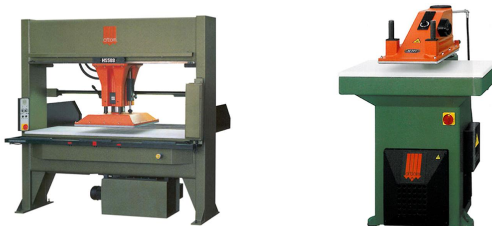
Figure 5. Different models of Hydraulic cutting machines. Source: CTCP
