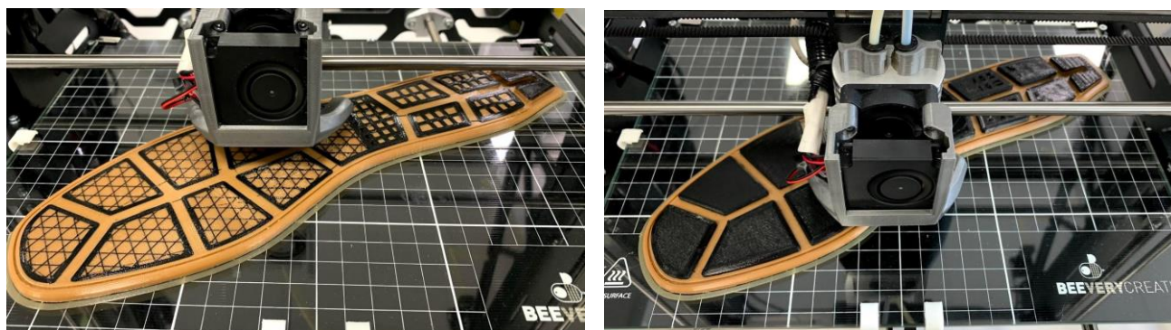
Figure 26. Printing a footwear sole. Source: CTCP
