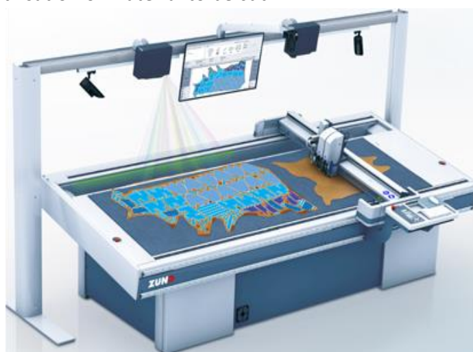
Figure 46. Automatic footwear cutting system. Source: CTCP
